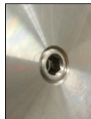
Set screw flush with surface
